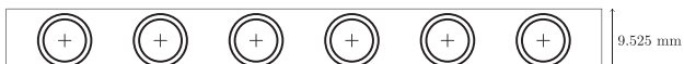
FIG. 2. Schematics of the “six-pack” sample holder. The top cylinder of each vessel is 7.9375 mm in diameter and 6.35 mm tall; the lower cylinder is 6.35 mm in diameter and 4.7625 mm tall. The total height of each vessel is 14.2875 mm.
