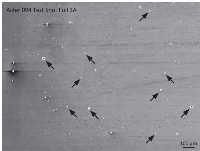
Figure 3. Secondary electron image of Acfer 094 test shot foil 3a showing representative craters.
